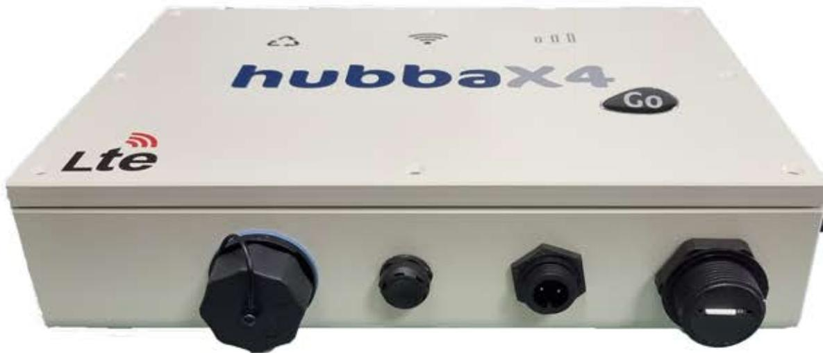
This single SIM powerful device comes in a bulkhead mountable IP66 rated enclosure with waterproof power and Ethernet connectors. It has status indicators and signal strength display and comes with our MIMO antenna system and two 8m cables.
